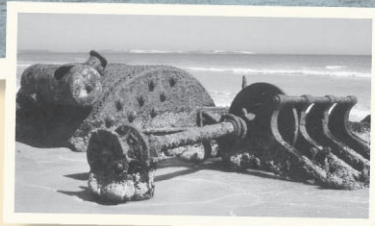
All that remains today: the Shannon's iron boiler and drive shaft. —KING ISLAND TOURIST DEVELOPMENT ASSOCIATION
